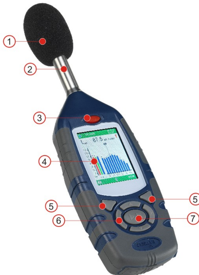
1 – Windshield (covering removable microphone), 2 – Fixed Pre-amplifier, 3 – ON/OFF Key, 4 – Display, 5 – Soft Keys, 6 – Navigation Cursor Keys, 7 – Run/Stop Key.
